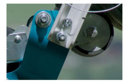
The hand brake is now applied. It must be checked whether the hand brake lever is at least two to three teeth away from the upper and lower stop. If this is not the case, the cable diameter must be readjusted.
