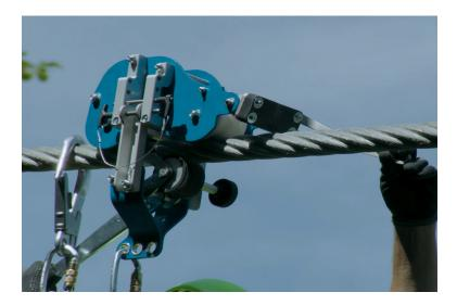
The dead man's brake must be held so far forward that it does not touch the cable. Its purpose is not to reduce speed. When travelling downhill, the dead man's brake must not be folded up completely.
