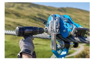
A cordless drill with the appropriate insert can be used for longer, flat rope sections and slight gradients.
