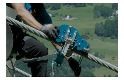
After the inspection, the carriage is fixed with the dead man's brake. The selfdriven carriage is now ready for travelling on the rope. The dead man's brake and braked back pressure roller prevent the self-driven carriage from driving away. Note: The back pressure roller can also be braked with the locking screw.
