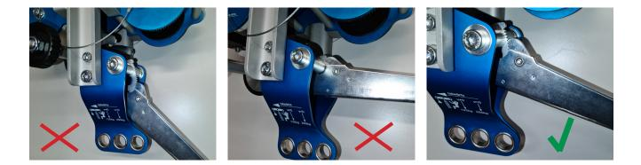
Before mounting the carriage, the length-adjustable fastener attached to the central fastening point (EN 813) should be mounted in one of the three positioning holes.
