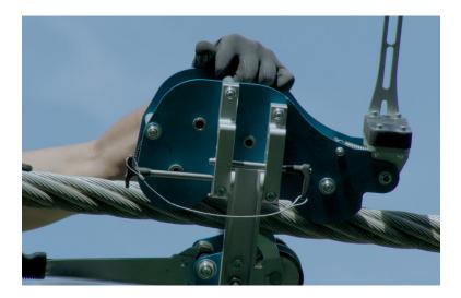
On the other side of the clamp, the self-driven carriage is tilted so that it can be folded up to the stop and secured with the quickrelease pin.
