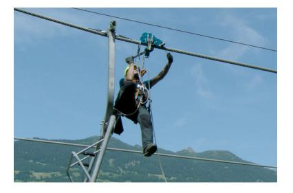
The rescuer attaches the hook of the longer lanyard to the rope behind the self-driven carriage and shortens the shorter lanyard up to the stop. The self-driven carriage is ready for travelling further.
